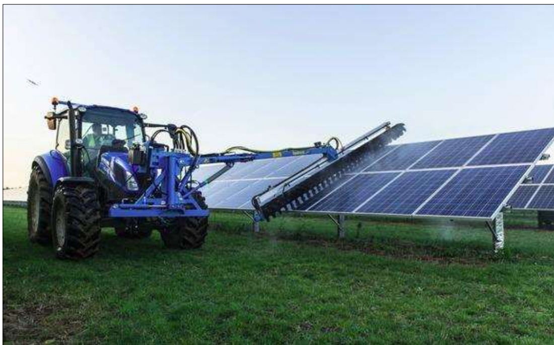
Figure 2-6: Tractor with module cleaning attachments
