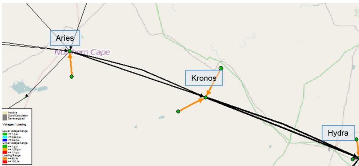
Figure 13: Reinforcements "Central" (orange: loading >80%, red: loading >100%)
